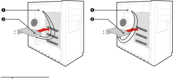
Figure 2–1 Possible Power Connection Locations on the Graphics Card
