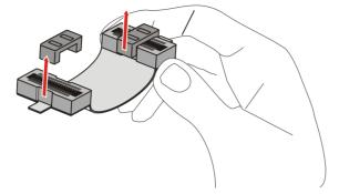
Figure 5–3 AMD CrossFire<sup>™</sup> Installation
