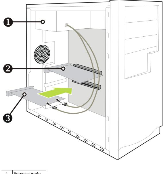
Figure 5–1 Connecting the Power Cables
